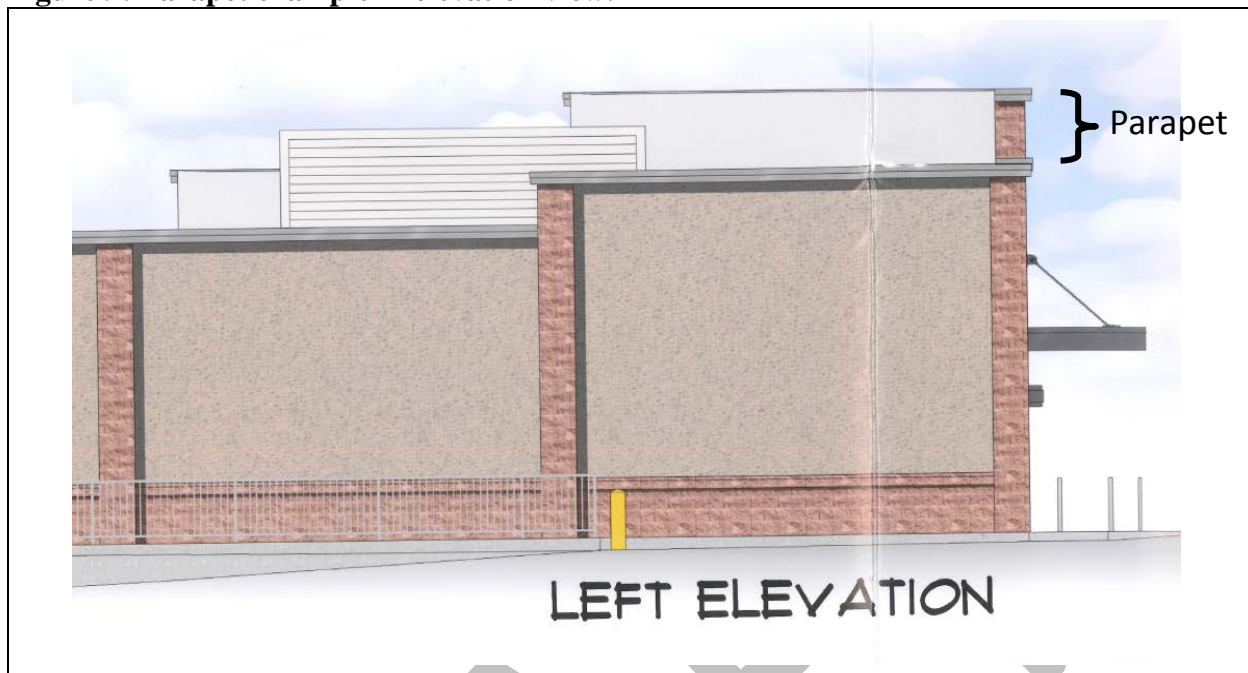
Figure 9: Parapet example in elevation view.
